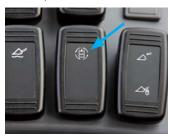
Aux hold switch: A simple push of the Aux hold switch sets and maintains the hydraulic oil flow for the implement. (All modes)
