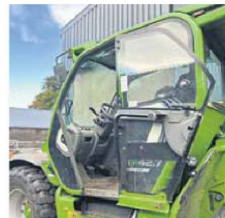
The ability to split and latch back the door is a major positive for Maurice.
