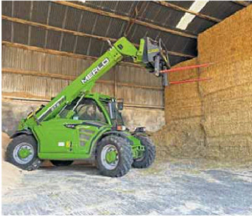
The P27.6 Plus has a maximum lift capacity of 2,600kg and reaches a height of 6m.
