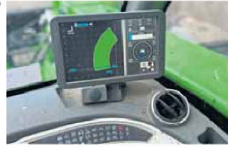
The TF42.7 has a built-in weight monitor, which displays the weight of the load placed on the headstock.
